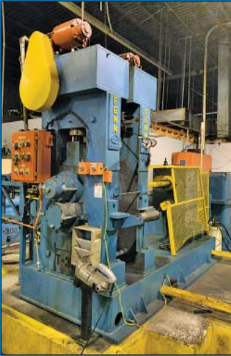
12" Fenn Rolling Mill w/ 150-HP Drive
